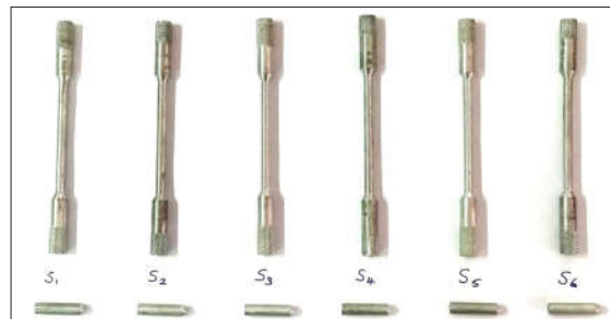
Fig. 3. Tensile and wear test samples
