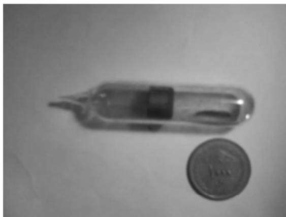
Fig. 1. Encapsulated sample by quartz before reaction in the furnace
