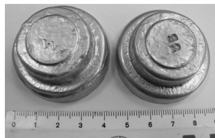
Fig. 1. Samples for testing the alloy porosity content
