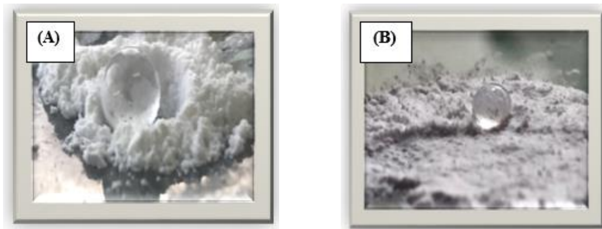
Fig. 3. The nano-silica powders hydrophobized by (A) ODTs and (B) HMDS
