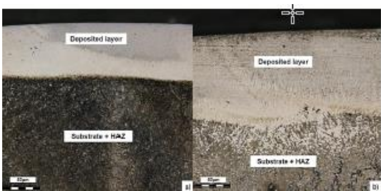
Fig. 8. Detail of WC-17Co deposited on AISI 4140 (a) and AISI H13 (b).
