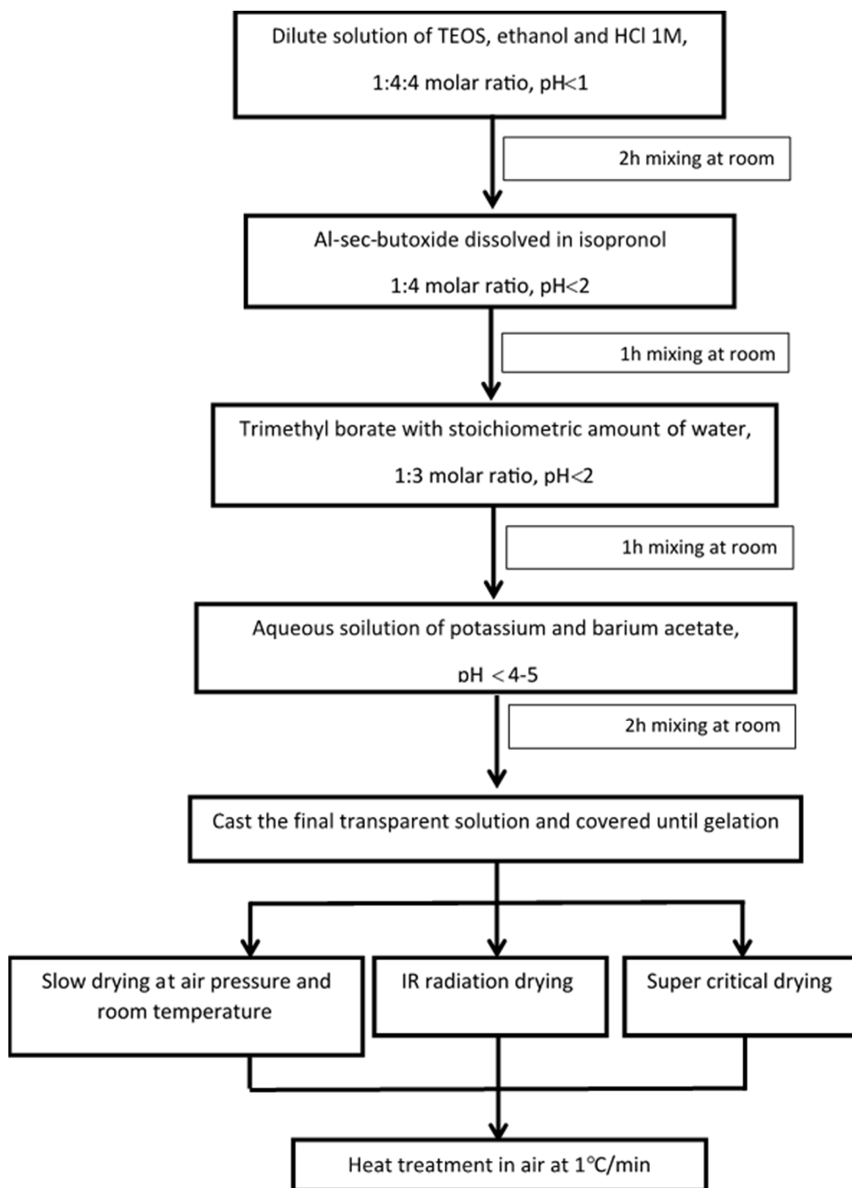
Fig. 1. Flow diagram of the chemical preparation procedures.
