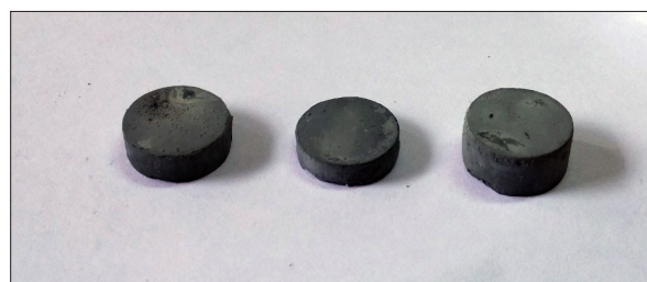
Fig.2. compacted pure silicon after pressing
