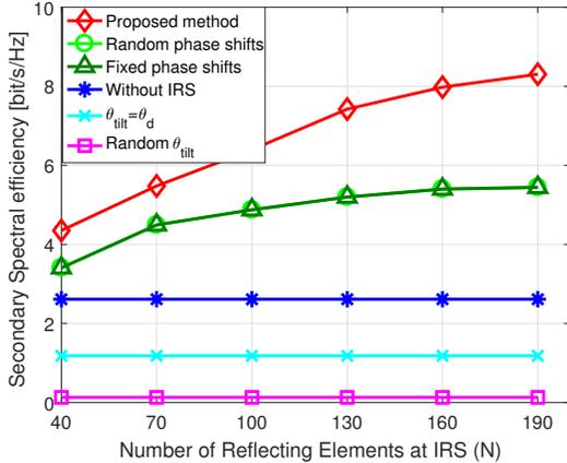
Figure 3. Secondary spectral efficiency versus the number of IRS elements ( $N$ ) (with  $P = 10\text{dBW}$ ,  $N_s = 2$ ).
