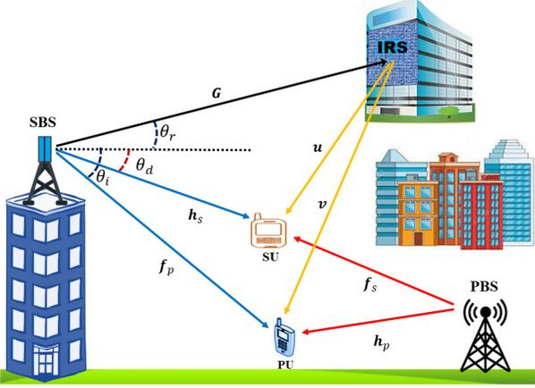
Figure 1. System model of the IRS-aided cognitive radio network.
