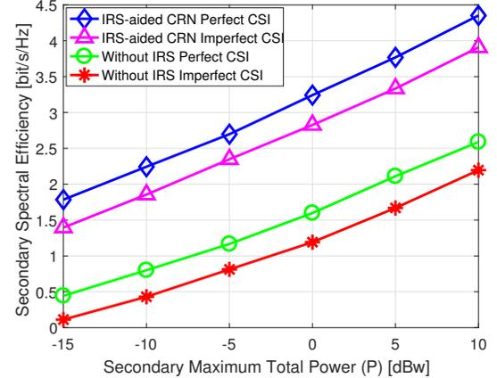
Figure 4. Secondary spectral efficiency versus the secondary maximum allowed total power ( $P$ ) (with  $N_s = 4$ ,  $N = 36$  and optimized tilt angle).
