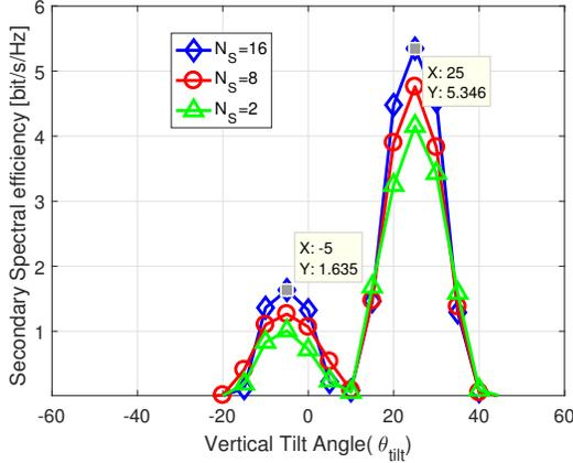
Figure 2. Secondary spectral efficiency versus the vertical tilt angle ( $\theta_{\text{tilt}}$ ) in different values of the number of antennas at the SBS ( $N_s$ ) (with  $P = 10\text{dBW}$  and  $N = 36$ ).
